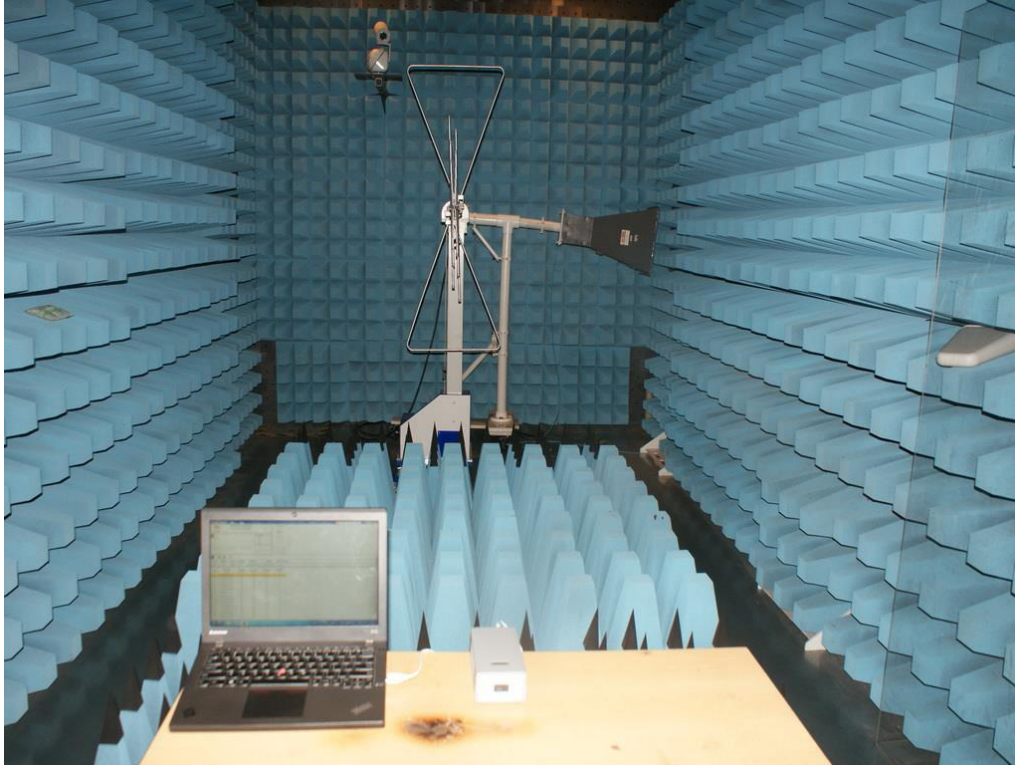
Photograph 4: Set-up for Radio-Frequency Electromagnetic Fields Susceptibility (RS) (Mode: A.2)
