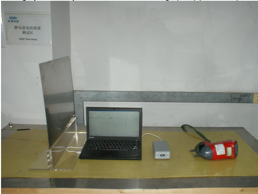
Photograph 6: Set-up for Electrostatic Discharge (ESD) (Mode: A.2)
