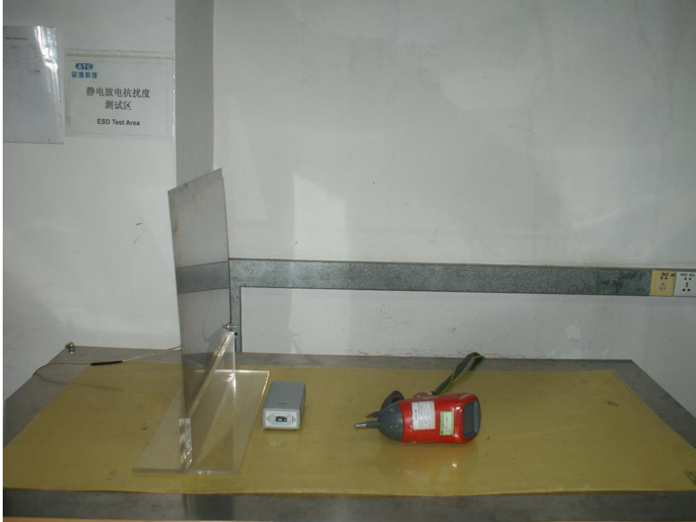
Photograph 6: Set-up for Electrostatic Discharge (ESD) (Mode: A.2)
