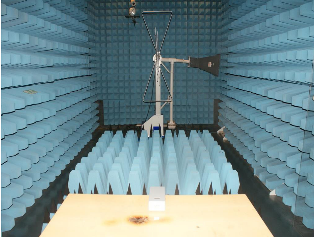
Photograph 3: Set-up for Radio-Frequency Electromagnetic Fields Susceptibility (RS) (Mode: A.1)
